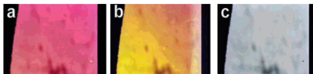
Figure 2. Homogeneously aligned nematic phase of 3a exhibits switching of colors with electric field (a) off and on at (b) 0.8 V \mu\text{m}^{-1} and (c) 2 V \mu\text{m}^{-1} at 155 °C. Horizontal edge is 0.75 mm.
